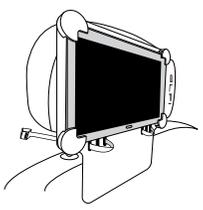
**8** Place the Alfi tablet assembly on the back of the passenger headrest making sure that each of the cable Ties go around each of the headrest Posts.
