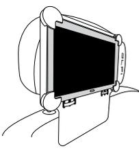
**10** Once both cable ties are installed, tighten each side equally. Make certain that the tablet mount is secure without excess slack in the cable tie.
