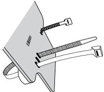
**5** Pass the second cable tie through hole **F** located on the right lower part of the mounting bracket, such that the cable tie head (locking end) is facing outward.
