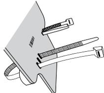
**6** Continue passing the cable tie from the front to the back of the mounting bracket, through hole **D**, until both ends are equal in length.
