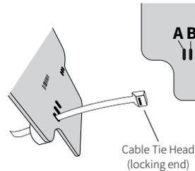
**3** Pass the first cable tie through hole **A** on the left lower part of the mounting bracket, such that the cable tie head (locking end) is facing outward.
