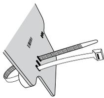
**4** Continue passing the cable tie from the front to the back of the mounting bracket, through hole **C**, until both ends are equal in length.
