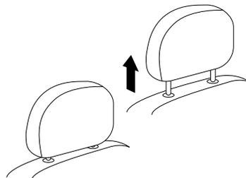
**7** Raise the passenger headrest until you have enough clearance to easily thread the cable ties through the gap between the headrest and the seat.
