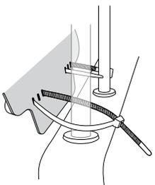
**9** Insert the tail of each cable tie into the cable tie head (locking end) and pull snug, leaving room for adjustment.
